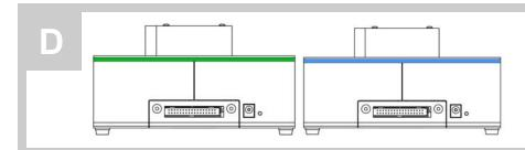
The LED strip around the base of the Quanser AERO should alternate between blue and green every 2 seconds.
