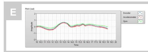
The **Pitch** (rad) graph should display the pitch angle measured through encoders (blue), accelerometer(red) and gyroscope(green).
