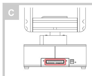
Using the NI myRIO MXP cable, connect the MXP A port on the NI myRIO to the QFLEX 2 myRIO connector socket on the Quanser AERO. Make sure the NI myRIO is connected to the computer via a USB cable and that the NI myRIO is powered.
