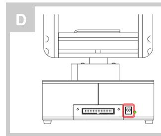
Connect the supplied 24V power supply to the Power connector on the Quanser AERO and to a wall outlet using the supplied power cable. The Power LED on the Quanser AERO should light up green.
